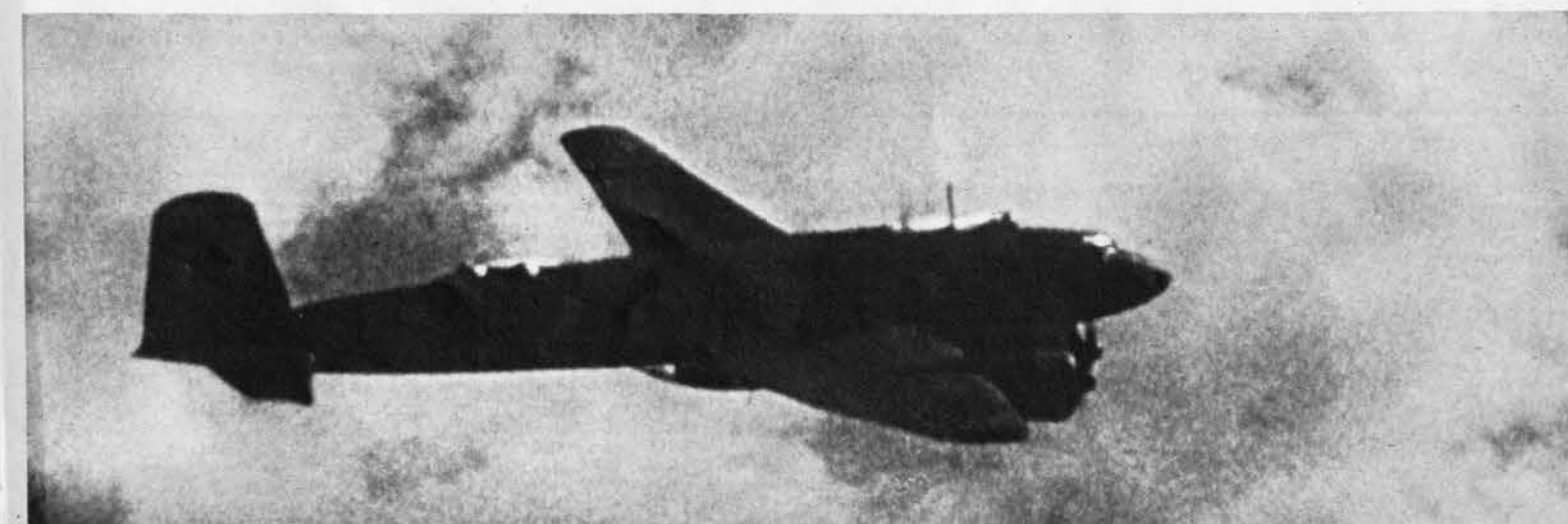
FW-200'S DORSAL LINE IS A SMOOTH CURVE BROKEN BY GUN BLISTERS ATOP CABIN AND AFT OF THE WING. WIDE, SQUARISH FIN RISES ABRUPTLY
